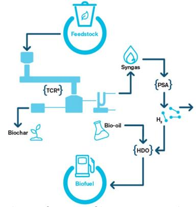
Thermo-catalytic reforming of biomass to produce synthetic transport fuels. Source: Fraunhofer Umsicht
